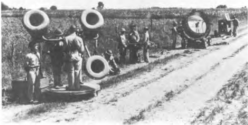
Antiaircraft sound-detection and searchlight equipment on maneuvers. (Courtesy of the Dwight D. Eisenhower Library.)
